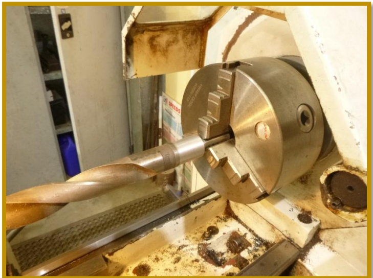
Jim T turns up the shank of a drill to fit a smaller chuck
