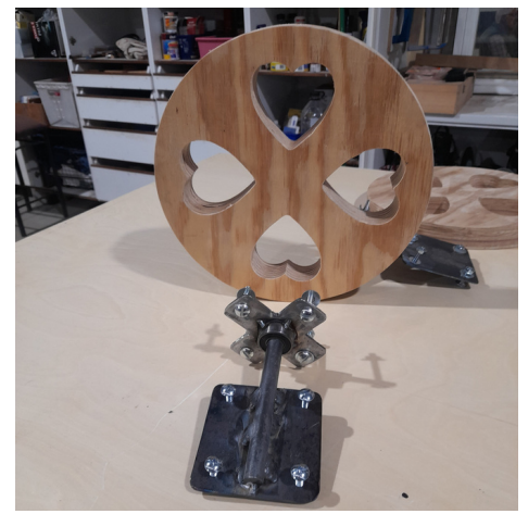
Wheel for flower cart with wheel & axle fittings welded by Ian A
