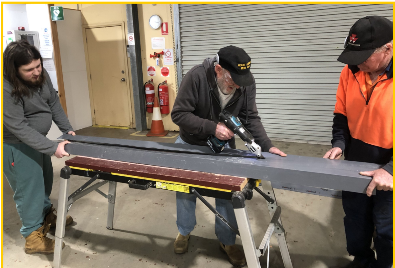
Stuart P & Dennis C holding bent metal while Frank McArdle cuts it to size for reinforcing corners on raised garden beds
