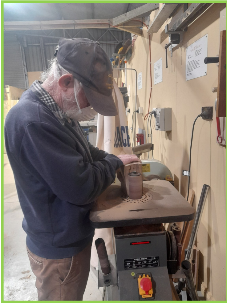
Glen B using vertical rotary sander to hollow out a rest for spectacles
