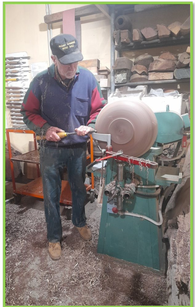
Don C turning a bowl on the wood lathe
