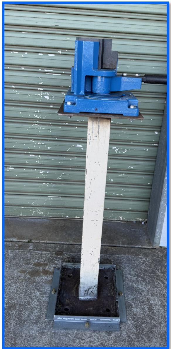
Permanent stand made for new heavy duty metal bender
