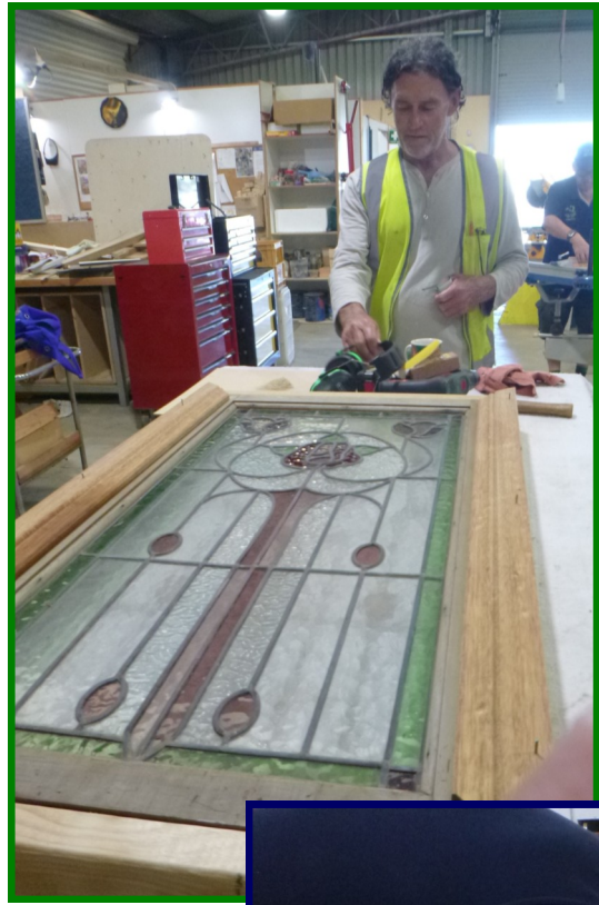
Ron P framing a stained glass window
