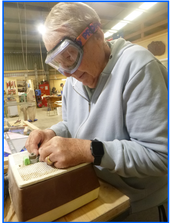
Graham T grinding a delicate glass curve for lead lighting
