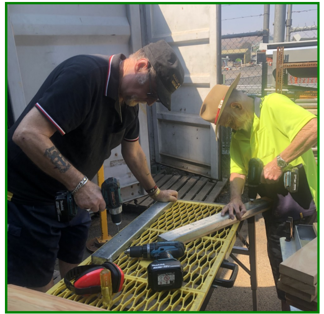
John K & Glen B using metal templates to drill 4 holes in each picket with hand drills
