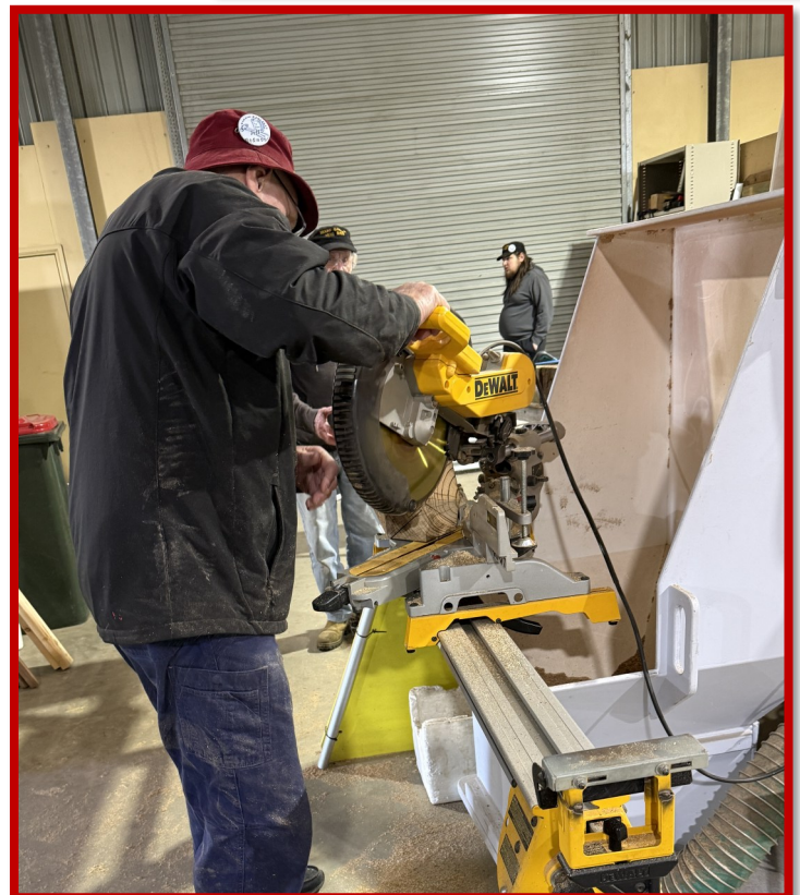
Jeff R cutting pointed tops on fence posts
